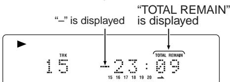
\* If **(TIME)** button is pressed when Super Audio CD disc that supports text is in use, time display is given priority and the text information will not be displayed afterward. To see the text information, press **(TEXT)** button.
