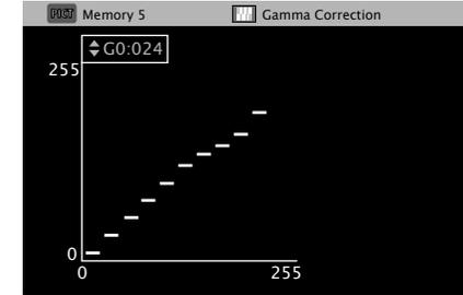
• On adjusting the brightness on the output side of bright parts on the disc side, the normally hard to see bright parts become clearly discernible images.
