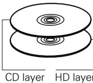
Two-layer Super Audio CD with an HD layer \* and a CD layer. The signals on the CD layer can be played on a regular CD player.
