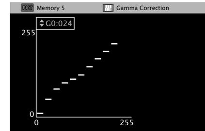
• On adjusting the brightness on the output side of dark parts on the disc side, the normally hard to see dark parts become clearly discernible images.
