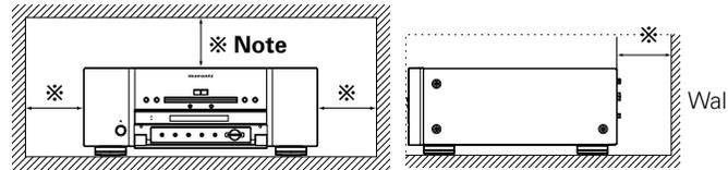
Do not place the UD9004 on an amp or other piece of equipment that generates heat.
