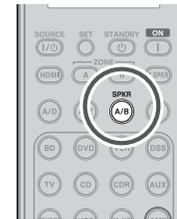
This unit has speaker system-A and speaker system-B for front L/R channels.
