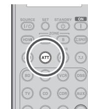
If the selected analog audio input signal is greater than the capable level of internal processing, the "PEAK" indicator will light up on the front display. If this happens, you should press the **ATT** button on the remote controller.
