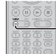
1. Press the **T.DISP** button 2 times to display the signal status.
