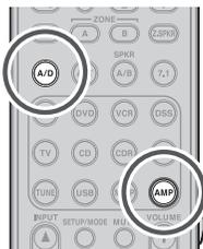
If you have already assigned the digital inputs, you can temporarily select the audio input mode for each input source as following procedures. Press the **AMP** button and press the **A/D** button. When this button is pressed, the input mode is switched in the following sequence. Auto → HDMI → Digital → Analog → Auto
