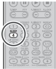
To program this unit for automatic standby, press the **SLEEP** button on the remote controller. Each press of the button will increase the time before shut down in the following sequence.
