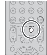
To temporarily silence all speaker outputs such as when interrupted by a phone call, press the **MUTE** button on the remote controller.
