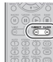
When the **◀▶** or **▶▶** button of the remote controller is held down during play, a search is started.
