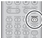
Each time the remote controller's **REPEAT** button is pressed, the modes are selected in the following order.
