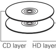
Two-layer Super Audio CD with an HD layer \* and a CD layer. The signals on the CD layer can be played on a regular CD player.
