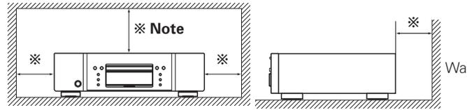
Do not place the UD8004 on an amp or other piece of equipment that generates heat.
