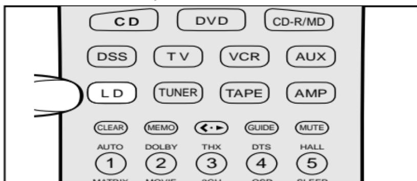
2. **LD** will be displayed on the LCD and the function codes will be set to operate the laser disc player, and if you double clicked the LD function button, the amplifier or receiver's input will be changed as well.
