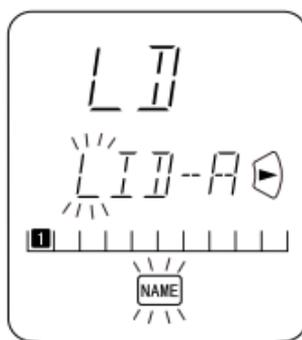
Once the desired character "L" appears, press either of the **<** or **>** Cursor buttons **(10)** and the L will be permanently written over the former character. Press the 0-key in order to replace unneeded extra characters with spaces ( $\frac{M}{M}$ ).
