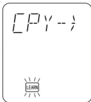
3. Select 1 of the LD function button on the copy source. Press the **LD function** button [8], and then press 1 on the **ten-key pad** [17] for 3 seconds.
