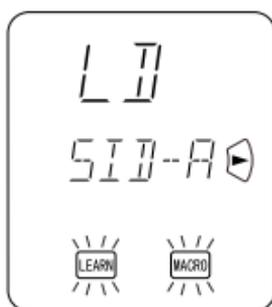
2. Press the **Function** button [8] for which you wish to program a series of operations. In this case, let's use the example of the laser disc player. Press the **LD Function** button [8].
