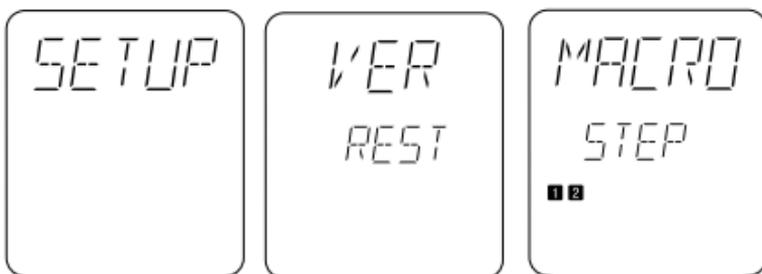
**VER: Switches the type of preset codes contained in the remote controller .**
