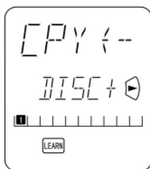
**CD** appears at LCD ②, and then the 1 (DISC+) characters stop blinking and remain lighted. (The Jog Dial name is displayed.)
