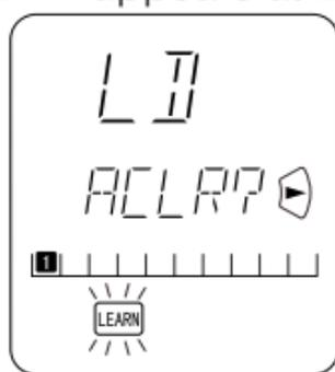
To go ahead with the clearing operation, release the buttons, and press the **OK** Cursor button **[10]**.
