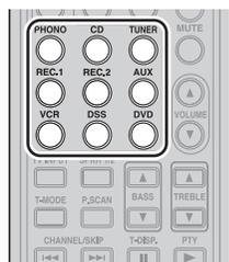
1. Select the input source to record by pressing the corresponding **input selector** button.
