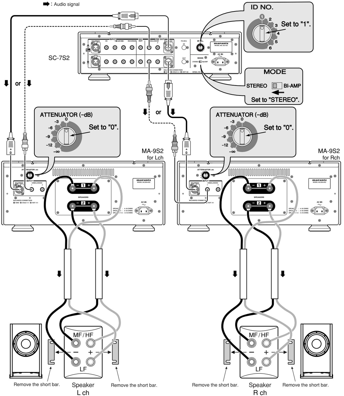
This connection can have options i.e. You may connect the units using either balanced or unbalanced cables.
