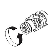
Turn counter-clockwise to loosen.
