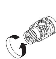
Turn counter-clockwise to loosen.
