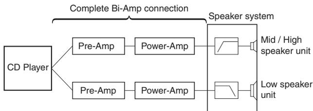
In this event, SC-7S2 is using as Monaural Amps. And separate Left/Right channels from the output terminal of CD players. As a result, influences between L channel and R channel Mid / High signal and Low signal will be eliminated. A maximum of 6 SC-7S2s, can be connected to each other, via remote cables.
