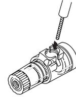
Insert conductor of cable.
