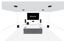
5.1.4: Regular 5.1 setup with 4 ceiling or 4 Dolby-enabled speakers
