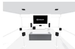
7.1.2: Regular 7.1 setup with 2 ceiling or 2 Dolby-enabled speakers
