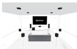
7.1.4: Regular 7.1 setup with 4 ceiling or 4 Dolby-enabled speakers
