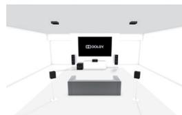
5.1.2: Regular 5.1 setup with 2 ceiling or 2 Dolby-enabled speakers
