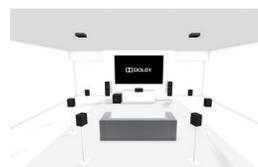
9.1.2: Regular 9.1 setup with 2 ceiling or 2 Dolby-enabled speakers
