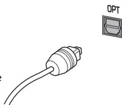
the protective shutter will open and you should hear it click into position when fully inserted. Be careful that you do not force the plug, because this could result in damage to the protective shutter, the cable, or the unit itself.
