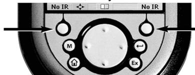
3. Press and hold either one of the **Left and Right Function** buttons, then tap the device you would like to jump to. No "input select" commands will be sent to your receiver/preamp.
