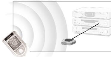
The RF signals sent out by the Remote Control are picked up by the RF-77 RF Extender. The RF Extender translates the RF signals in IR signals and sends the IR signals to the appropriate device. Therefore, the RF Extender has to be placed near the device you're operating with the RF Extender's sending eye pointed to the device.
