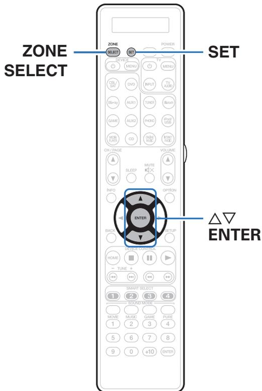
When the ZONE SELECT is pressed, only the set zone can be operated with the remote control unit.
