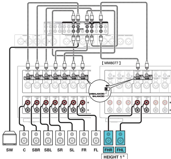
\* The rear height speakers can be connected instead of the front height speakers. In this case, set the height speakers to be connected under "Height" - "Layout" in the menu. (🔗 p. 243)
