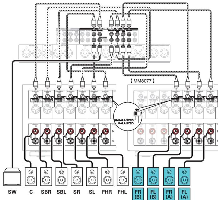
\* The height speakers, ceiling speakers and Dolby Atmos Enabled speakers can be connected to the HEIGHT1 speaker terminals. Set the speaker to be connected from "Height" - "Layout" in the menu. (📖 p. 243)
