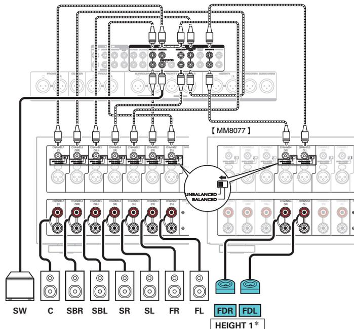
\* The surround Dolby speakers can be connected instead of the front Dolby speakers. In this case, set the Dolby Atmos Enabled speakers to be connected under "Height" - "Layout" in the menu. (👉 p. 243)
