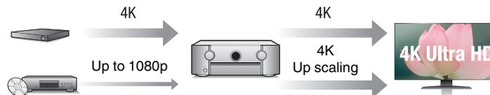
This unit is equipped with a 4K video upscaling function that allows analog video or SD (Standard Definition) video to be output via HDMI at 4K (3840 × 2160 pixels) resolution. This function enables the device to be connected to a TV using a single HDMI cable, and produces high definition images for any video source.
