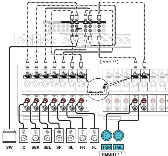
\* The top front or top rear speakers can be connected instead of the top middle speakers. In this case, set the ceiling speakers to be connected under "Height" - "Layout" in the menu. (☞ p. 243)
