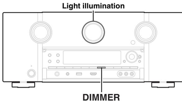
You can switch the light illumination around the main display on or off. The default setting is “On”.
