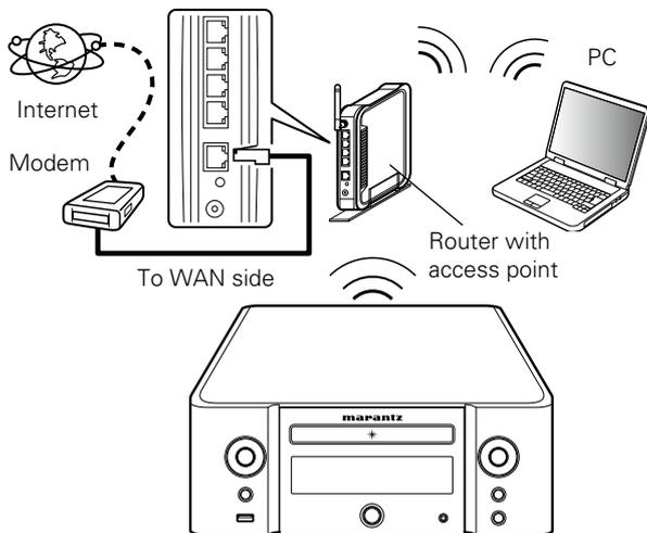
\* This unit comes with a built-in Wi-Fi antenna.
