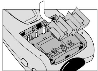
3 Insert four AA batteries as indicated on the bottom of the battery compartment.
