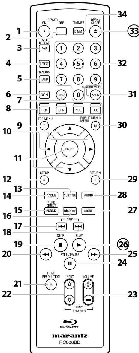
The unit can also be turned on by pressing the buttons with circled numbers.
