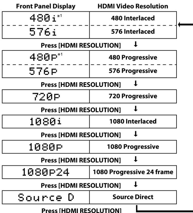
\*1 "480i" and "480p" will be displayed only when an NTSC disc or a1080p/24 frame material is being played back.
