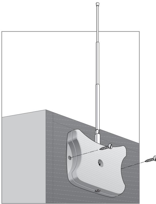
**Tip** Depending on the surface, it may be possible to attach the Receiver unit to the furniture using a piece of 2-sided tape or velcro. Find the right position and make sure there is sufficient space.
