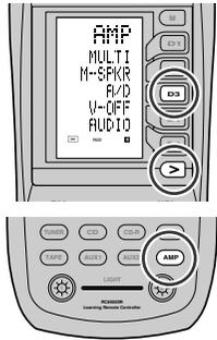
If you have already assigned the digital inputs, you can temporarily select the audio input mode for each input source as following procedures. Press the **AMP** button and press the **>** button until PAGE4 is displayed. Press the **A/D (D3)** button. When this button is pressed, the input mode is switched in the following sequence.
