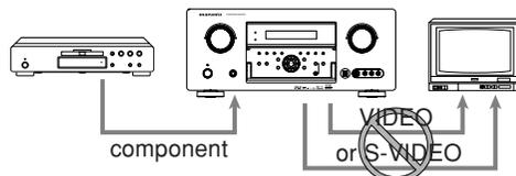
The signal cannot be converted from the component to the video or S-video.
