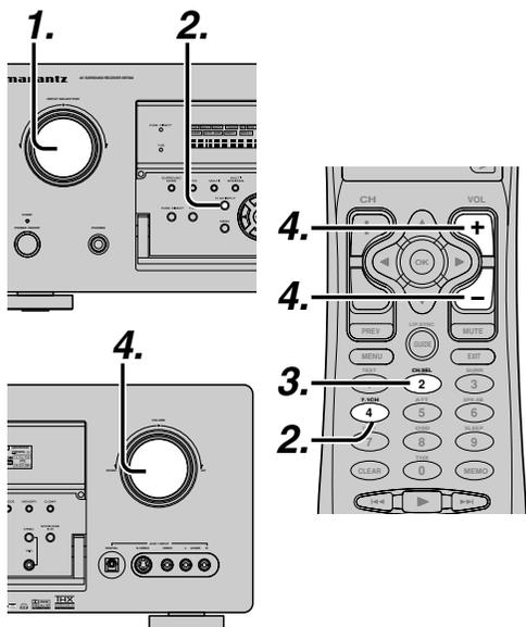
1. Select a desired Video source to decide the routed video signal to the **Monitor Outputs**.
