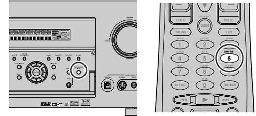
SR7500 has speaker system - A and speaker system- B for front L/R channels. You can select these systems by pressing **SPEAKERS A/B** button on the front panel or **SPK-AB** on the remote.
