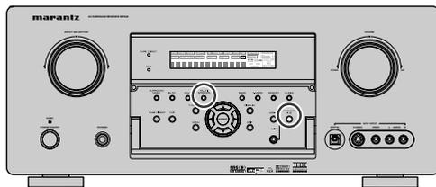
Should the operation or display seem to be abnormal, reset the unit with the following procedure. The SR7500 is turned on, press and hold the **MULTI + SPEAKERS A/B** buttons simultaneously for 3 seconds or more. Remember that the procedure will reset the settings of the function selector, Surround mode, delay time, TUNER PRESET etc., to their initial settings.
