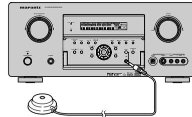
2. Set the microphone at ear height as in the actual listening position. Use a stand or tripod to position the microphone.
