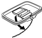
3. Insert the hook at the bottom of the loop part into the slot at the base part.
