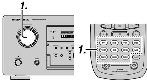
1. Select the input source to record by turning the **INPUT FUNCTION SELECTOR** knob on the front panel or simply press the **input selector** buttons on the remote.
