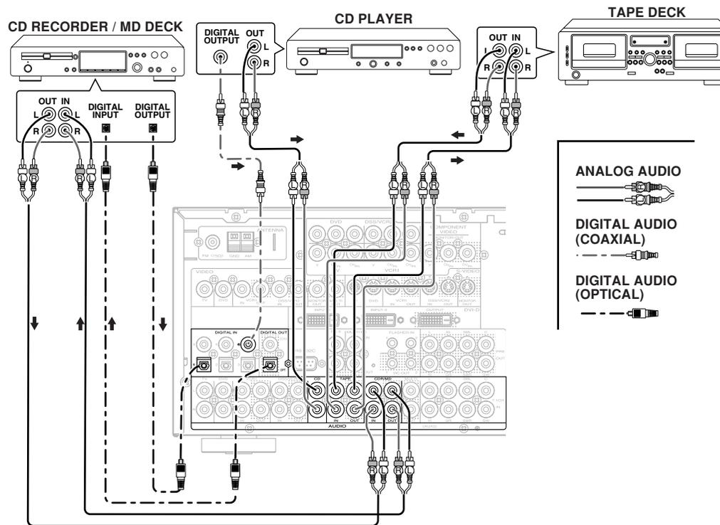
The output audio signal from the TAPE OUT jack and the CD-R/MD OUT jack is the same signal which is currently selected.
