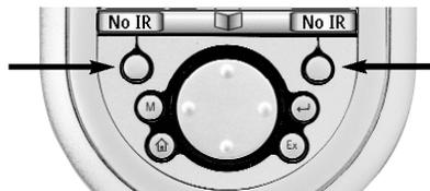
3. Press and hold either of the two **Left** and **Right Function** buttons, then tap the device you would like to jump to. No “input select” commands will be sent to your receiver/preamp.
