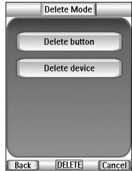
Note By pressing the “Undo” function button, the button you just deleted is restored.
