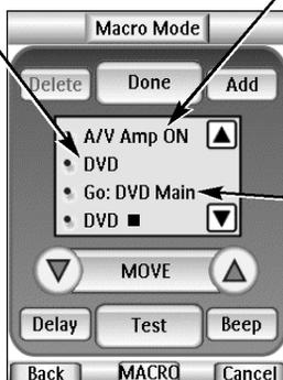
**AMP - ON** - When a device name and a button name are listed, that particular button's IR command will be issued.
