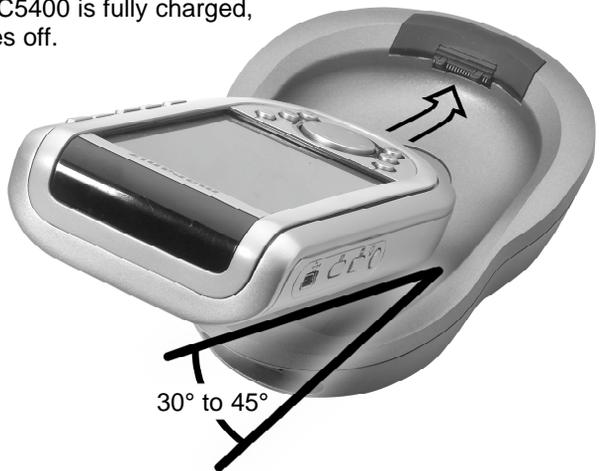
Make sure you lift the RC5400 up at an angle of 30° to 45° when you take the RC5400 out from the docking station.
