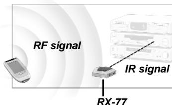
Your devices will always receive IR signals either directly from the RC5400 or from the RX-77.
