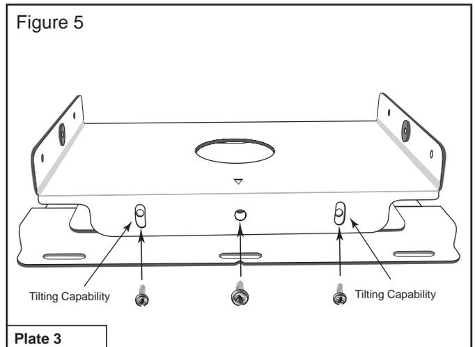
The newly combined Plate 3 provides 10° degrees of horizontal tilt. When positioned, tighten with screws provided.
