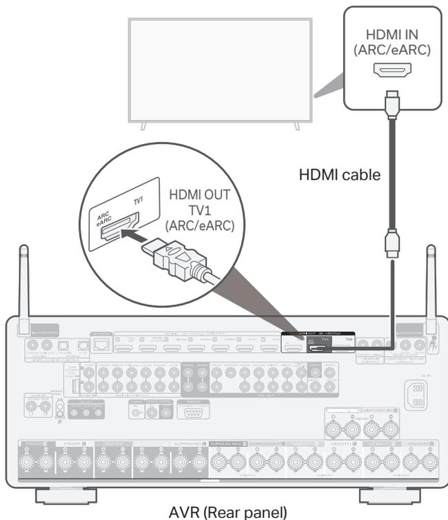
Using a high quality HDMI cable\*, connect one end to the HDMI port labeled “eARC” or “ARC” on your TV. Connect the other end to the HDMI OUT TV 1 port on your AVR.
