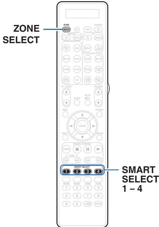
Settings such as the input source, volume level and sound mode can be registered to the SMART SELECT 1 - 4 buttons.
