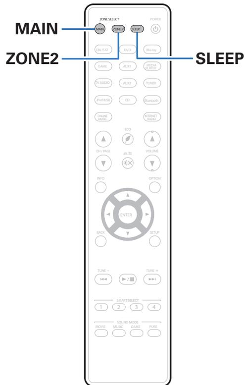
You can have the power automatically switched to standby once a set time has elapsed. This is convenient for viewing and listening while going to sleep. The sleep timer function can be set for each zone.
