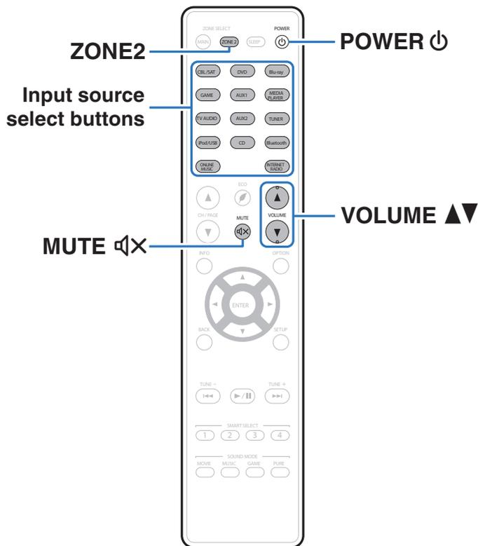
**1 Press ZONE2 to set the operating zone to ZONE2 with the remote control.**
