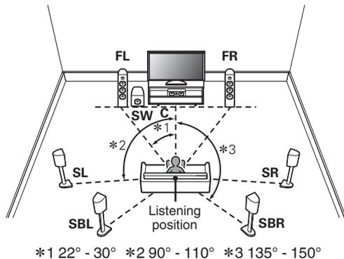
■ When 5.1-channel speakers are installed
