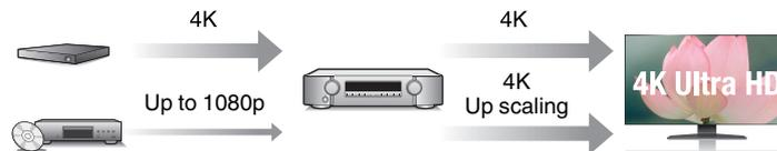
This unit is equipped with a 4K video upscaling function that allows SD (Standard Definition) video to be output via HDMI at 4K (3840 × 2160 pixels) resolution. This function enables the device to be connected to a TV using a single HDMI cable, and produces high definition images for any video source.
