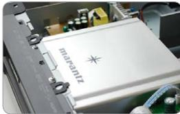
Fully Shielded Mechanism
