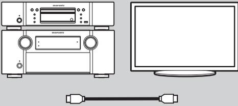
Connect this unit and a television or an AV receiver using an HDMI cable.
